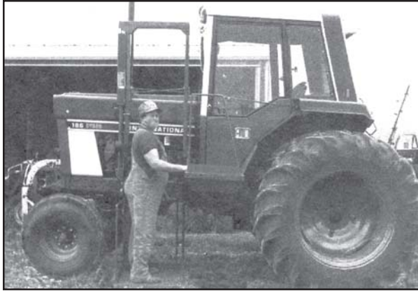
Figure 18. Chip outfitted his International 186 with a standing platform left after his injury.
