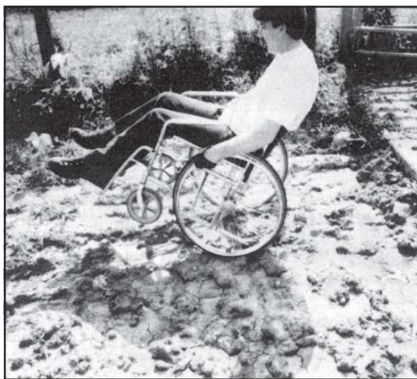
Figure 9. It appears that most farmers using wheelchairs prefer the lightweight, sports-type chair with pneumatic tires and inserts to reduce the frequency of flat tires.
