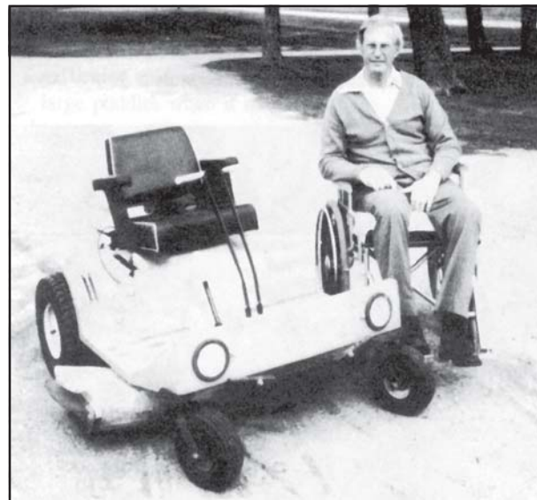
Figure 13. Some lawn and garden equipment is hand-operated and provides a way to both mow the lawn and travel around the farm.
