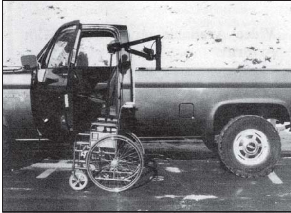
Figure 14. On most farms, the pickup truck is the most important means of transportation. In some cases, it is considered a mobile office. Here a hoist has been mounted in the bed of the pickup to lift the chair for storage.
